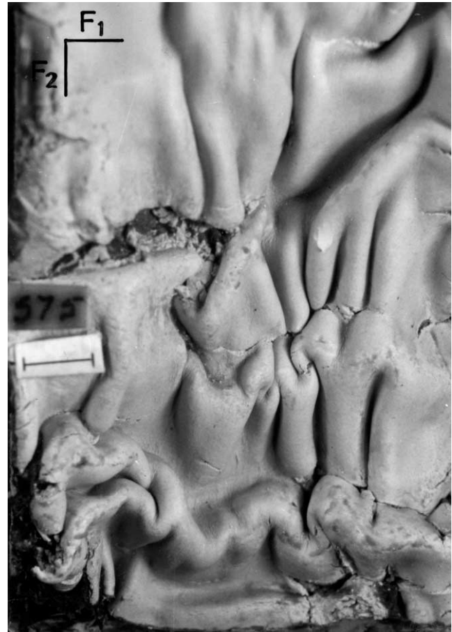
Fig. 14. Superposed buckling with an inclined enveloping surface. The F_1 folds were horizontal with P_2 parallel to the F_1 -axes. The enveloping surface is inclined towards the viewer with a dip of 68^\circ . In the central part, the F_2 and the F_1 folds are subparallel and their interference has produced non-planar sheath folds. Scale bar is 1 cm.
